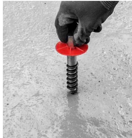
Option 1 – The quick anchor is simply pressed into the fresh concrete. The required concrete cover is achieved through adjustment of the anchor plate.
